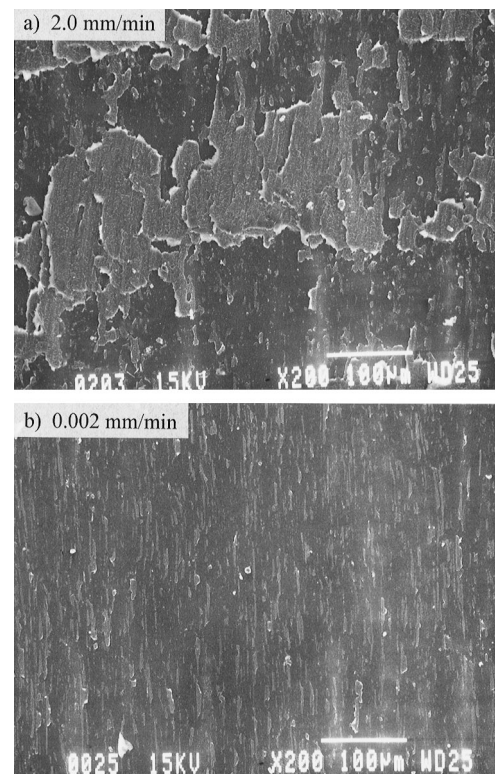
Fig. 3. Scanning electron micrographs of the PC fracture surface at two peel rates. The crack propagated from left to right.
